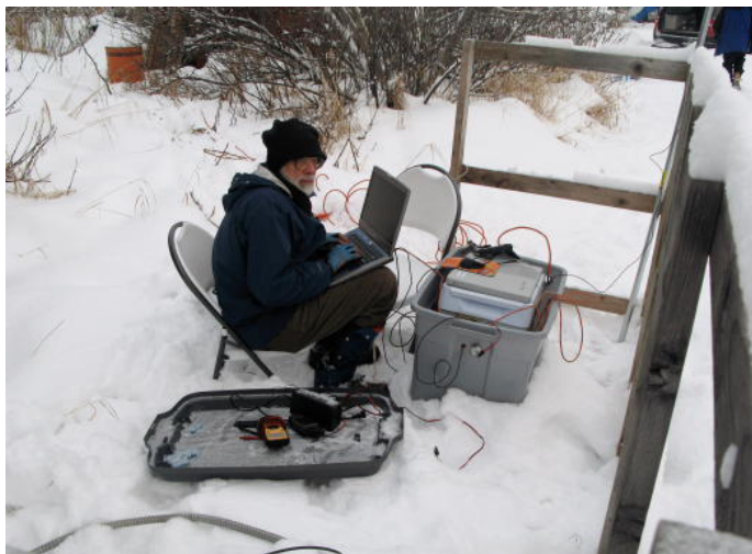
Setting up portable mapping stations on Kenai Peninsula coast overlooking Cook Inlet, used to study Redoubt Volcano eruptions. Above: Paul Krehbiel working on station electronics. Right: Ron Thomas setting up VHF receiving antenna. Redoubt is in background obscured by ever-present clouds.
