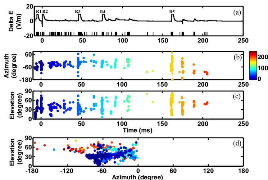
*Radiation during a multi-stroke CG flash at 15:45:35 on July 19th, 2009: (a) fast electric field waveform recorded by the fast antenna, (b) azimuth angle of sources versus time, (c) elevation angle of sources versus time, (d) radiation source location.*
