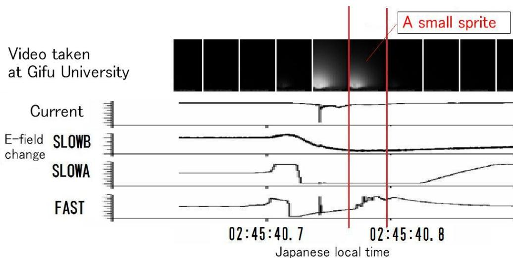
*A small sprite and the electric current and electric field changes of the lightning discharge that likely produced the sprite. All the data are synchronized with time.*
