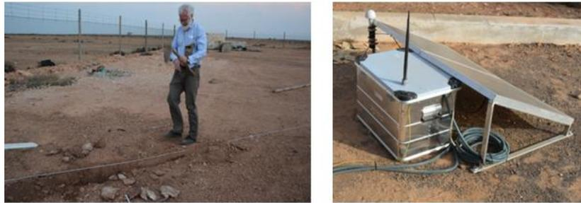
Fig. 2 Earle Williams during the antenna alignment (Left) and outdoors sensor electronics powered by solar panels (Right).
